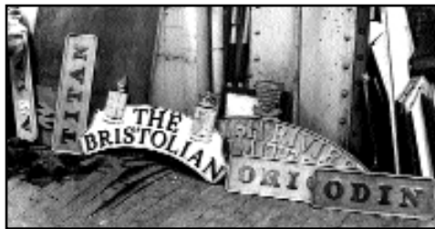
For many years before Newton Replicas became the main supplier of nameplates, the foundry at Swindon Works was the producer. This picture shows some of the wooden patterns in the Swindon foundry, mainly for the 1960s cast Type 4 plates, plus the headboard for 'The Bristolian'. JS
